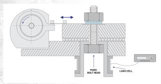
TEC Series wedge locking washers have been tested on a Junker Vibration Machine. The Junker test, according to DIN 65151, considered the most severe vibration test for bolted joints, is used to determine the point at which a bolted joint loses its preload when subjected to shear loading due to transverse vibration.
