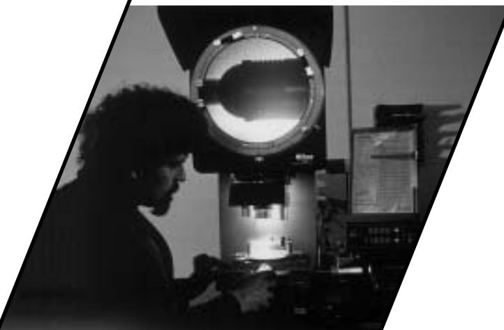
Profile Projector – Measuring Instrument for in-process control of production.
